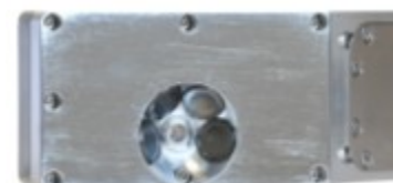
4 sensor circular through hole focused array SDD
